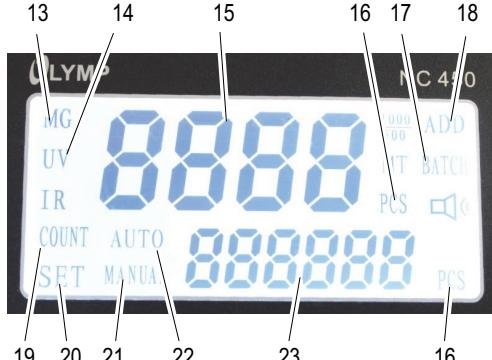
The diagram illustrates the display during the power on self-test. Some of the features illustrated do not belong to the functional range of this bank note counter.
