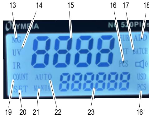
The diagram illustrates the display during the power on self-test. Some of the features illustrated do not belong to the functional range of this bank note counter.
