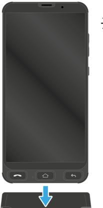
Insert the smartphone in the charging cradle with the charge contacts (3) facing down.
